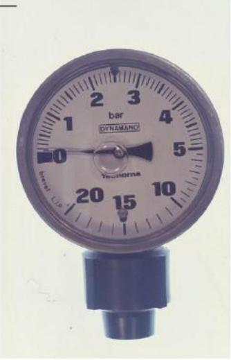
4.5.5 For analogue pressure gauges the minimum diameter of the pressure gauge cases shall be 63 mm.
