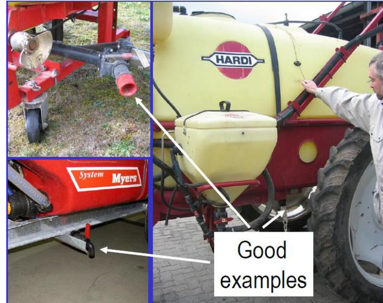
**4.4.5** There shall be a clearly readable liquid level indicator on the tank which is visible from the driver's position and from where the tank is filled.
