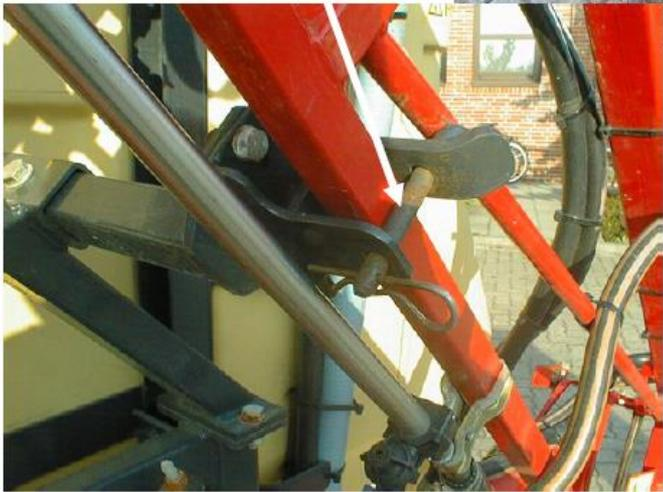
**4.8.3** The boom shall be securely lockable in the transport position.
