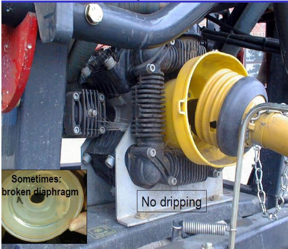
**4.2.4** There shall be no leakages (e.g. dripping) from the pump.
