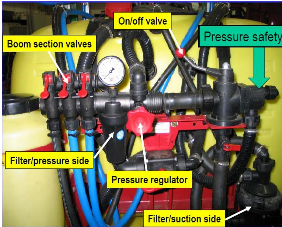
**4.2.3** When there is a pressure safety valve on the pressure side of the pump, this valve shall work reliably.
